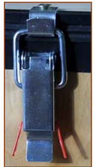
Cover lock with protector (prevents from unintended opening and indicates, that negative is loaded)
