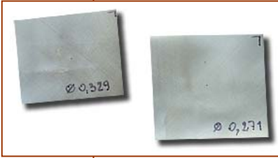
Apertures made from thin aluminum plate (beer can used). There are holes in center :- ) and size written (mm).
