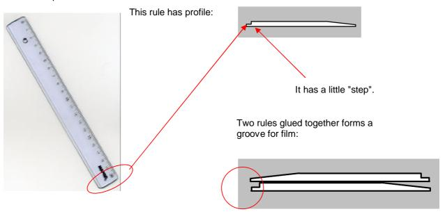
I used this groove for film holding. Two rails with film loaded:
